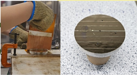
1st soldering (the upper surface)
