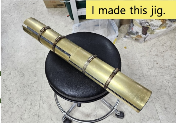
Roll it up and tighten it with a clamping jig
