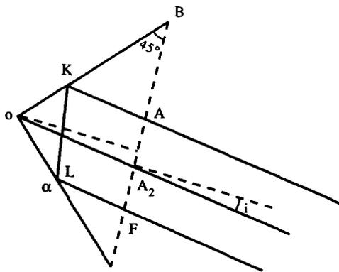
Figure 2 Paths of the rays in a rectangular dihedral reflector
