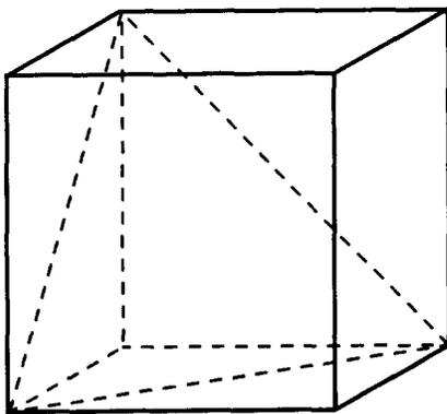
Figure 3 Intersection of a cube for the creation of a trihedral rectangular reflector
