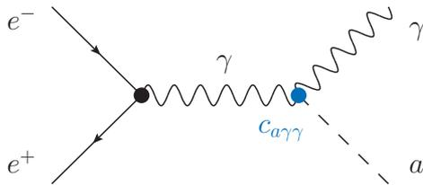
$$\sigma_{\text{NR}}(s) = \frac{\alpha_{\text{em}}}{24} \frac{c_{a\gamma\gamma}^2}{f_a^2} \left(1 - \frac{m_a^2}{s}\right)^3$$
