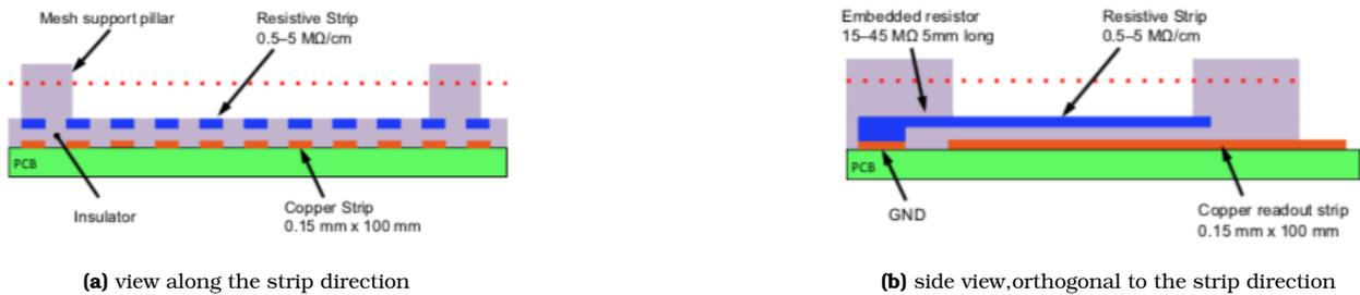
**Figure 7:** Sketch of the detector principle (not the scale), illustrating the resistive protection theme
