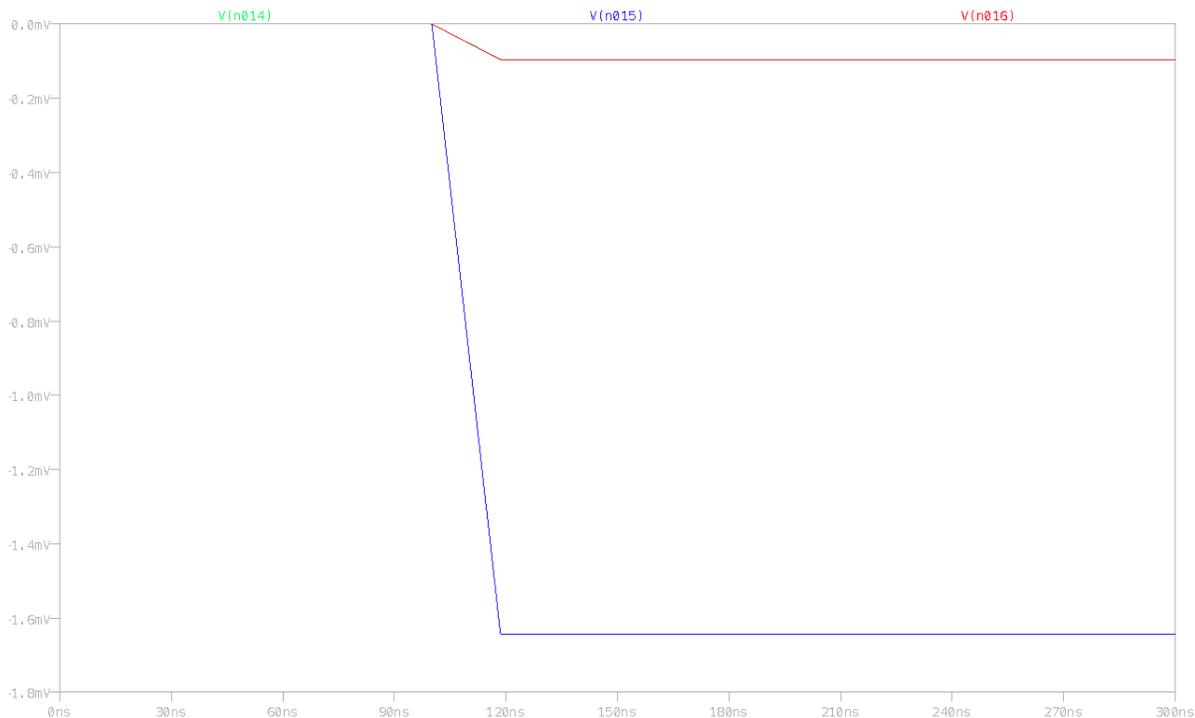
Figure 66: output voltage for central and neighbor strips
