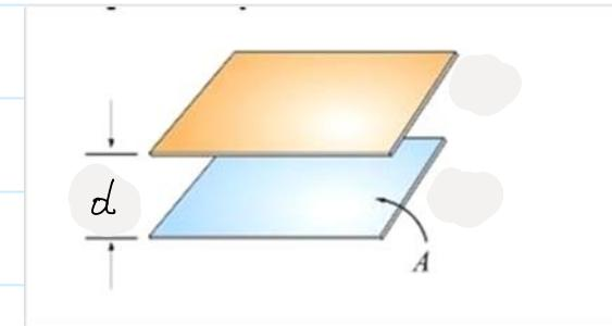
2 perfectly conducting parallel plates : set-up of
